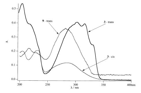
Fig. 4. UV absorption spectra of compounds 3-trans, 3-cis and 9-trans dissolved in n-hexane. Vibrational structure, appearing as broad peaks or shoulders in the spectral region 250–350 nm, is found for compounds with planar geometry (such as 3-trans) only. Peak maxima in this spectral region shift to shorter wavelength as the molecular structure changes from planar(3-trans) to nonplanar (3-cis and 9-trans). Spectra were recorded for  $1 \times 10^{-4}$  M solutions in 1 cm wide cuvettes.
