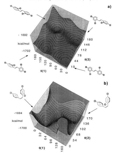
Fig. 1. Potential energy surfaces for: (a) the *trans* isomer of molecule **6**; and (b) the *cis* isomer of molecule **5**. Potential energies as functions of the dihedral angles  $\theta(1)$  ( $C_6-C_1-C_7-C_8$ ) and  $\theta(2)$  ( $C_7-C_8-C_1-C_{6'}$ ) (see Scheme 1). Semi-schematic molecular conformations corresponding to the potential minima are also shown.
